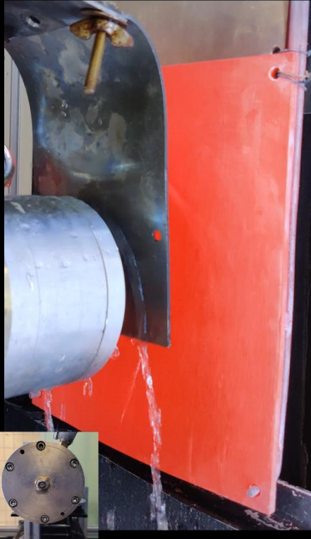
Nickel, s=5 mm, 0 mm/sec, 1.18 L/min, ( p= 5 bar), 1X Fulljet nozzle, d=1.05 m
