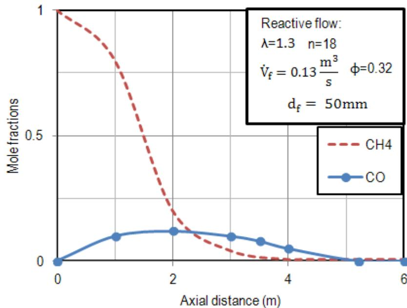
Figure 8 : CH4 and CO profiles in axial distance.
