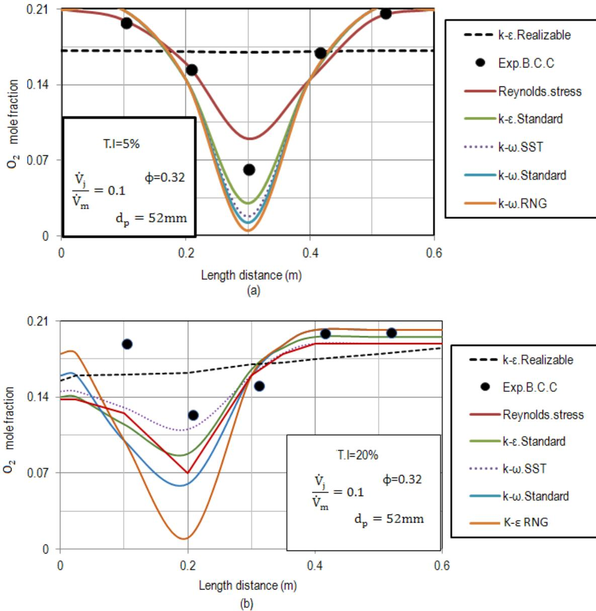
Figure 3: Oxygen profile for comparison for different turbulence models and validation
