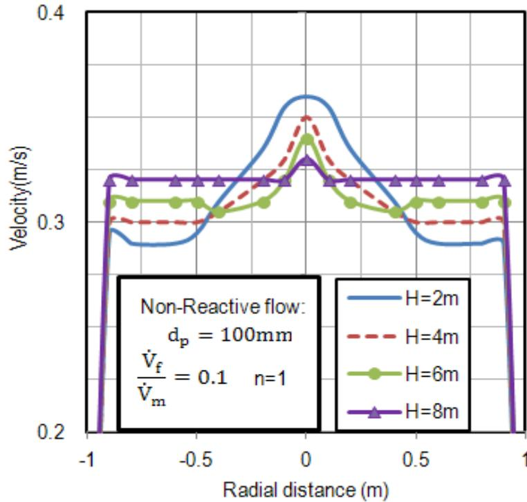
Figure 4: Velocity profile at different heights at  $\phi=0.32$ .
