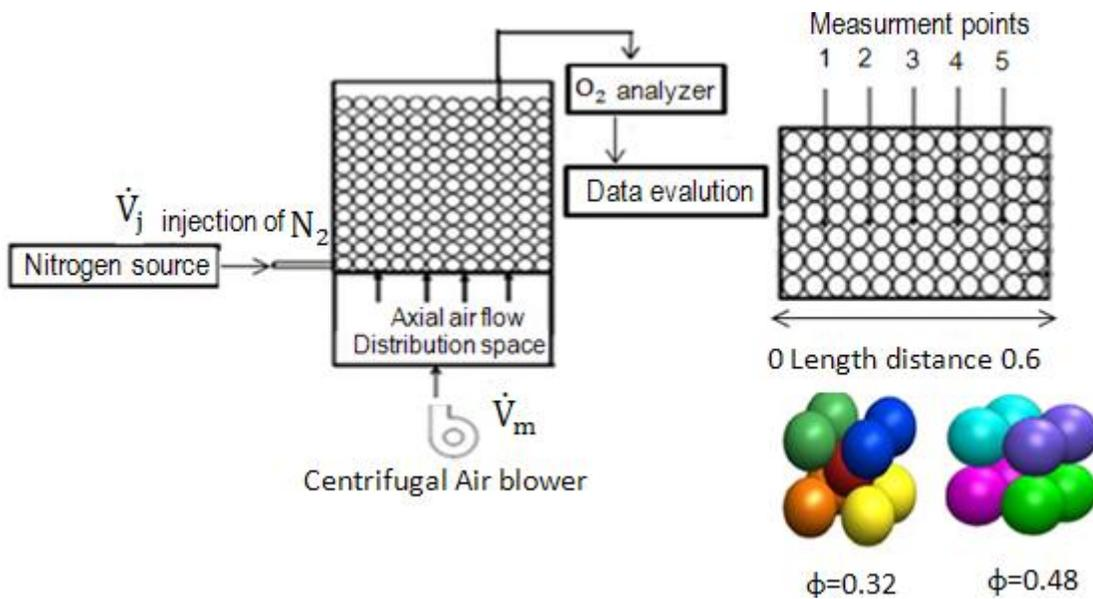
Figure 2 : Schematic description of the experimental setup.
