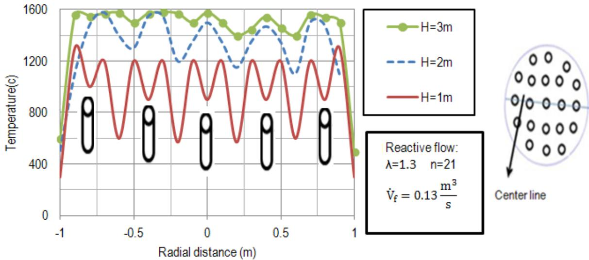
Figure 7: Temperature profiles at different heights when  $n=21$ .
