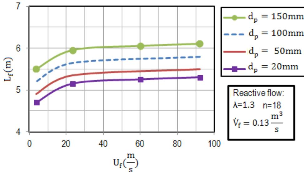
Figure 9 : Influence of fuel velocity on the flame length.
