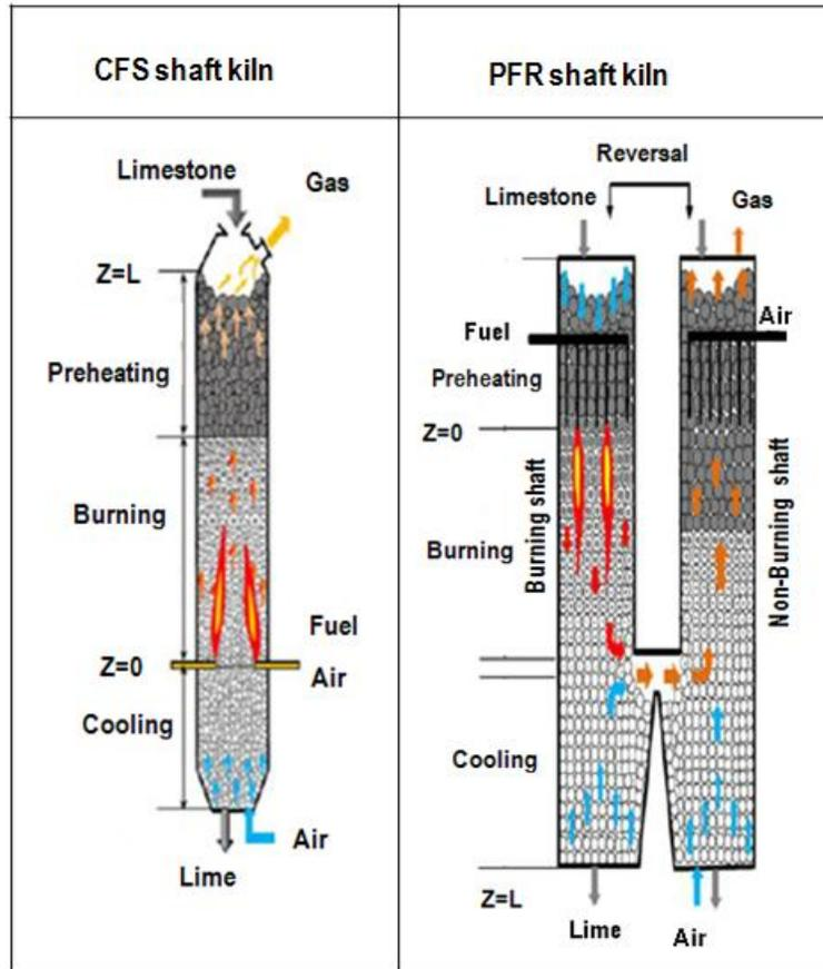
Figure 1: Schematic design of a CFS (a), and a PFR lime shaft kiln(b).
