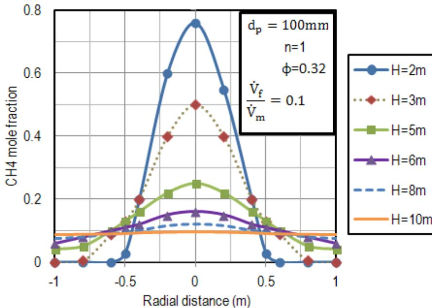
Figure 5 : Fuel distribution at different heights.
