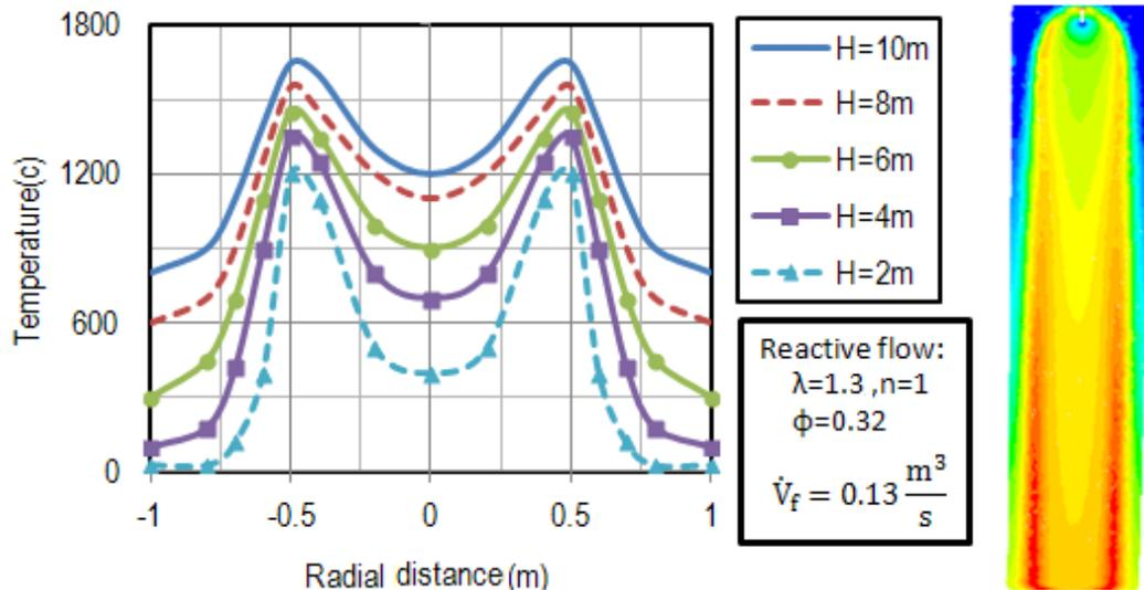
Figure 6 : Temperature profile at different heights.
