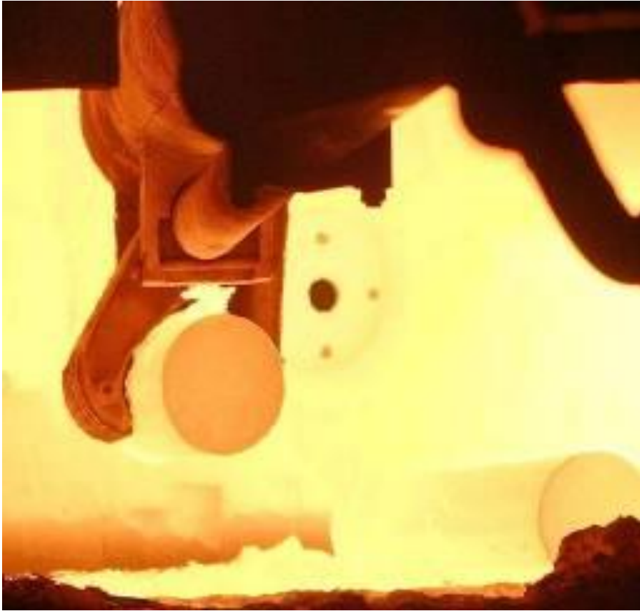
Natural Gas fired Flameless Oxyfuel at Rotary Hearth Furnace for Tube Production at ArcelorMittal
