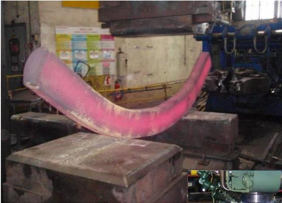
Fertiger Spant (25 kg)
