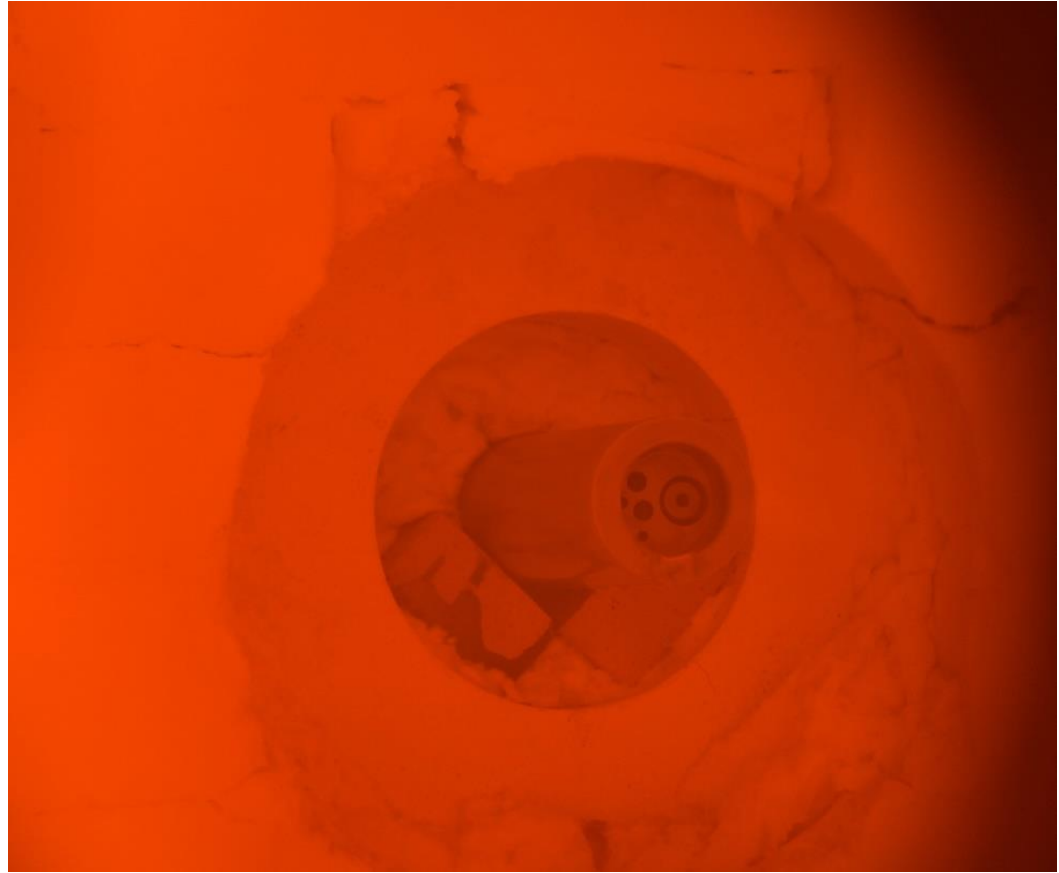
Hydrogen fired Flameless Oxyfuel at a Linde Technology Centre, Stockholm
