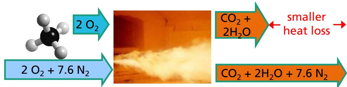
■ thermal integration for T<sub>waste gas</sub> > 850 °C
