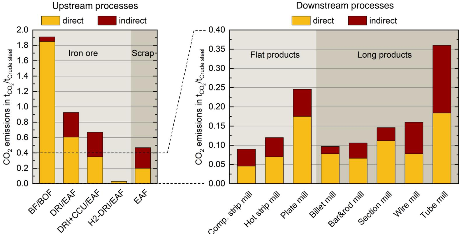
Data from: E. Malfa: Sustainable heating technologies for today's and tomorrow's metal industry, dissHEAT workshop at ESTAD 2023, 15/06/2023, Duesseldorf based on EUROFER, Determination of GHG emissions in energy-intensive industries, 2020; ENERGIIRON process data, 2015; Internal Tenova evaluations, 2022. CO<sub>2</sub> intensity for grid electricity 0.376 t/MWh
