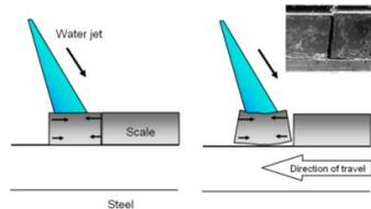
Differential Thermal Contraction  $f(\text{time, scale thickness/diffusivity, etc.})$
