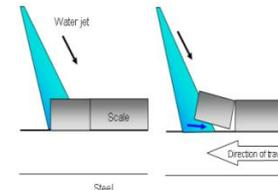
Shear at Scale - Steel Interface
