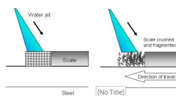
Mechanical Impact  $f(P, \text{nozzle}) \Rightarrow \text{Impact pressure IP}$
